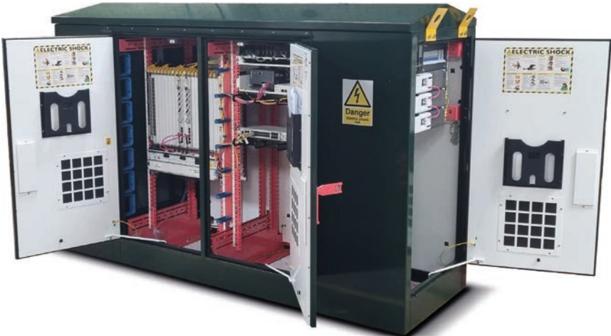
IMAGE LEFT SHOWS: Cannon DEKA Integrated Multi-Bay Cab with UPS L-ION Battery(s), Rectifier 48VDC Distribution, Fibre splice management, client NOKIA FX16, ADVA, FORTINET equipment installed, cabled, configured (IP address etc), firmware updates and fibre spliced.
