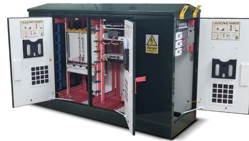
IMAGE LEFT SHOWS: Cannon Integrated Multi-Bay Cab with UPS L-ION Battery(s), Rectifier 48VDC Distribution, Fibre splice management, client NOKIA FX16, ADVA, FORTINET equipment installed, cabled, configured (IP address etc), firmware updates and fibre spliced.
