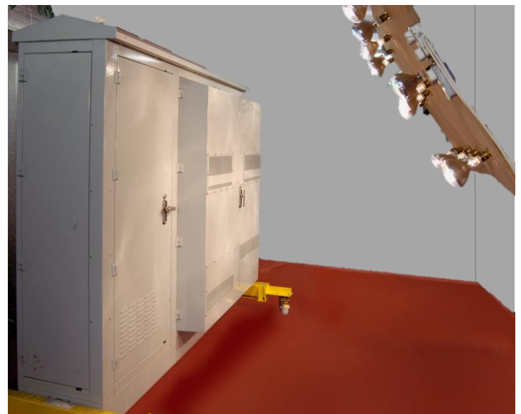
Chamber capable of maintaining air temperatures above the local ambient up-to a maximum 60°C with a solar gain of 1.1kW/m 2
